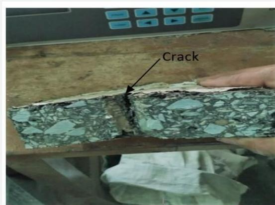
Figure 6: Cracked specimens.
